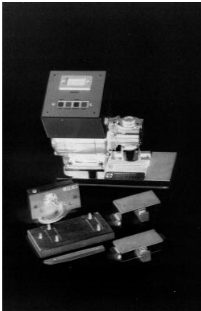
FIG. 1 Sutherland Rub Tester and Attachments
